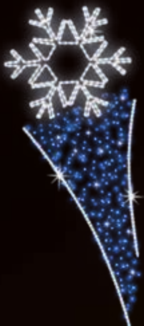
POL-1204 3D decoration – 250x100 cm cone – cool white snowflake, cone's inner parts in blue colour. LED ornament to be placed on a lantern – 250x100 cm with connecting wires and installation elements. The decoration is based on aluminium chassis in the shape of cone, welded using the TIG method from 20/20/2 and 20/10/2 rectangular moulding.
